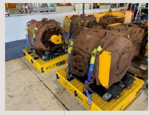
DAYWALK worked with the client to design, certify and manufacture an Australian-made transport system for the wheelsets and traction motors that were to be transported. The design incorporated two parts, a logitics-engineered, adjustable frame design and reusable covers for sustainable preservation.
