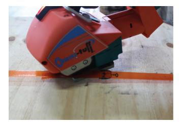
Clench the lever to release strap from tool. Slide tool away from strap in a sideways motion.
