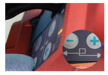
Adjust tension – press plus for higher tension (LED light moves higher up the bar)
