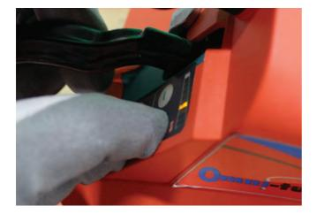
Adjust weld intensity – Press top plus button to increase weld (LED light moves up the bar)
