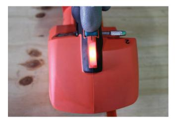
Hold down Button 1 to tension strapping. Release when desired tension is reached.
