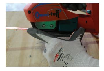
8. Ensure strapping is aligned under the Feedwheel.
