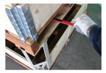
4. Insert tail end of strap through the pallet- a strapping lance is recommended.
