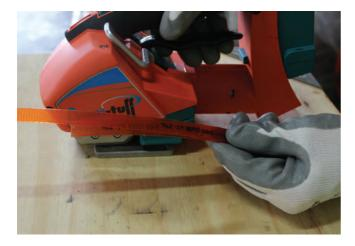
6. Ensure tail end of strap is underneath coil end of strap.
