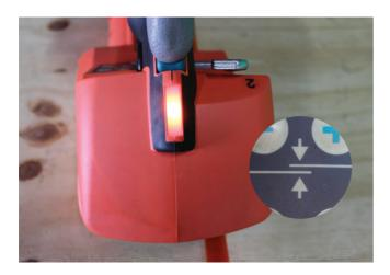
Ensure large orange light is on (either flashing or solid orange). If light is not on, push the large black tension button (with a 1 on it) for a split second.
