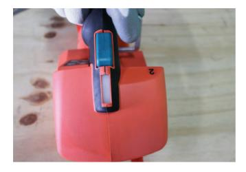
Pull back Weld Lever (2) to weld and cut strap. Note: Do not release the Feedwheel until the beep has sounded.
