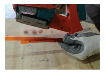
7. Clench lever to release Feedwheel and insert the strapping.
