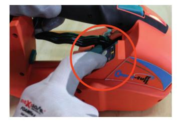
Hold down the two plus buttons for approximately 10 seconds, until the LED light shines.
