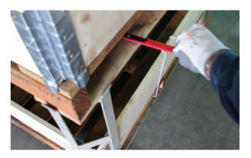
**4.** Insert tail end of strap through the pallet - a strapping lance is recommended.
