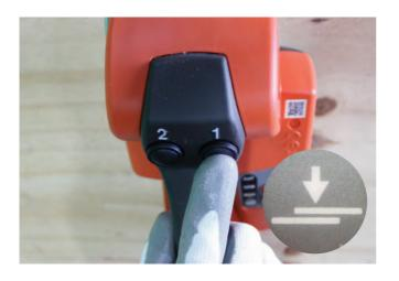
1. Switch on tool by pressing the number '1' button once. Machine will beep and green LED will flash.
