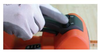
Press button 1 again for one second. This activates the tension and welding function.
