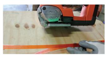
**7.** Place tail end of strap is underneath coil end of strap.
