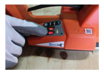
2. Hold down weld adjustment button until the illuminated numeral flashes.
