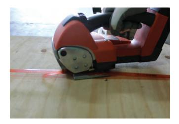
**3.** Clench the lever to release strap from tool. Slide tool away from strap in a sideways motion.
