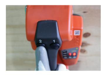
2. Press button 2 to complete welding and cutting of strap; a beep signals completion of process. Note: Do not release the Feedwheel until the beep has sounded.
