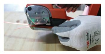
**8.** Clench lever to release Feedwheel and insert the strapping.
