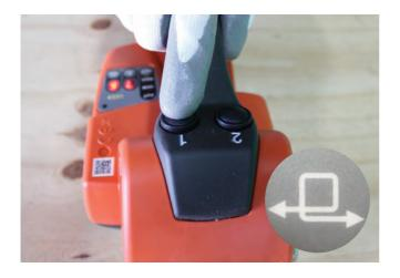
1. Switch on tool by pressing the number '1' button once. The machine will beep, and green LED will flash.
