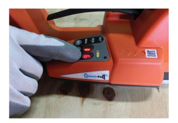
2. Hold down tension adjustment button until the illuminated numeral flashes.
