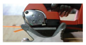
**9.** Ensure strapping is aligned under the Feedwheel and Welding Group.
