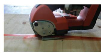
Clench the lever to release strap from tool.Slide tool away from strap in a sideways motion.
