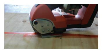
2. Clench the lever to release strap from tool. Slide tool away from strap in a sideways motion.
