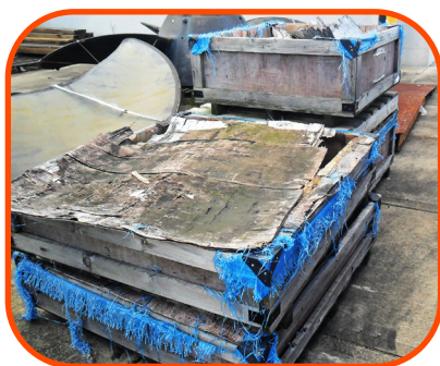
Broken frames used for the propeller were not sufficient fo the scope of the component.
