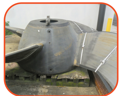
Errorded timber pallet providing minimal support to a propeller with high risk of damage occuring.
