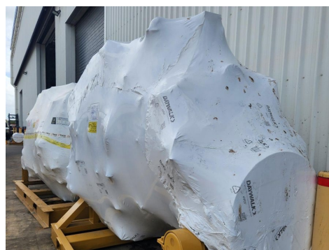
eVCI film after extended outdoor exposure — still fully sealed and legible
