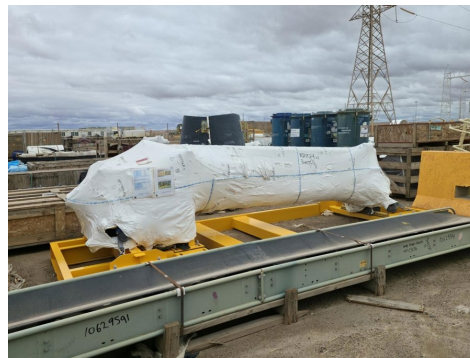
Long-term outdoor storage — eVCI wrap holding up in an exposed mine site yard
