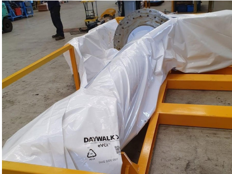
eVCI film applied to a complex component profile
