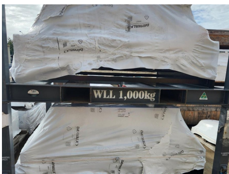
Liebherr components individually eVCI-wrapped and racked for transit
