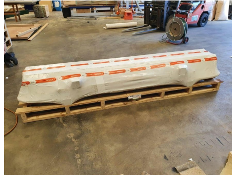
Long-profile steel bundles fully encapsulated in eVCI film
