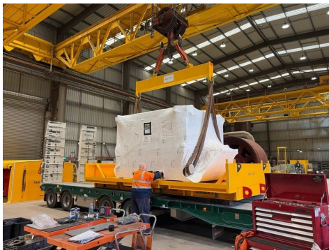
Crane-lifting a fully eVCI-wrapped motor onto a Daywalk Transporta frame
