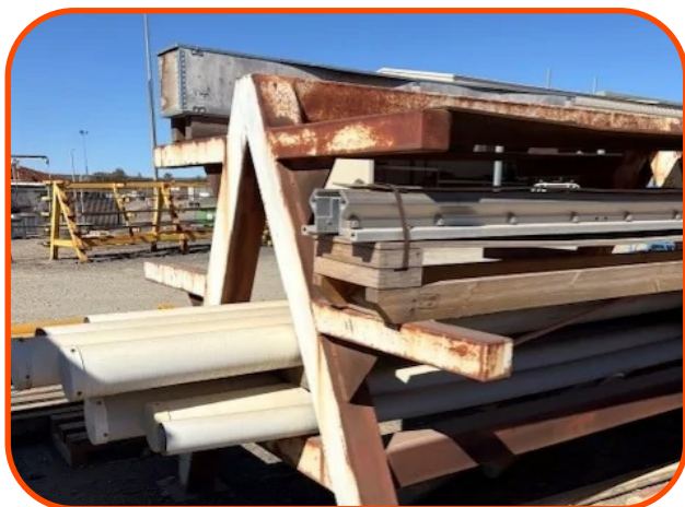
Old racking was showing signs of age including rust, damage and general wear and tear.
