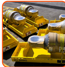
Cylinders of various types, sizes and capacities transported and stored safely on pre-engineered frames.
